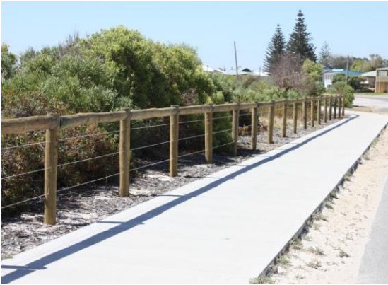
Treated pine post and rail with cable ($50 m 2 )
